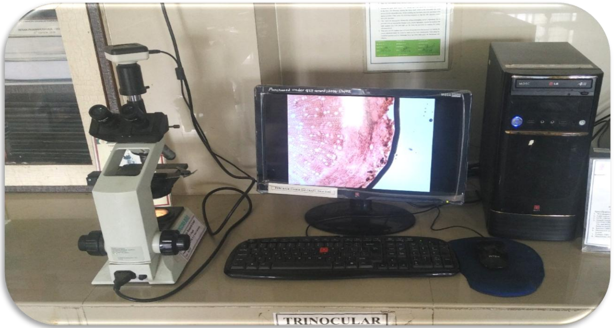
Trinocular microscope attached to digital camera and the image is analyzed by computer
